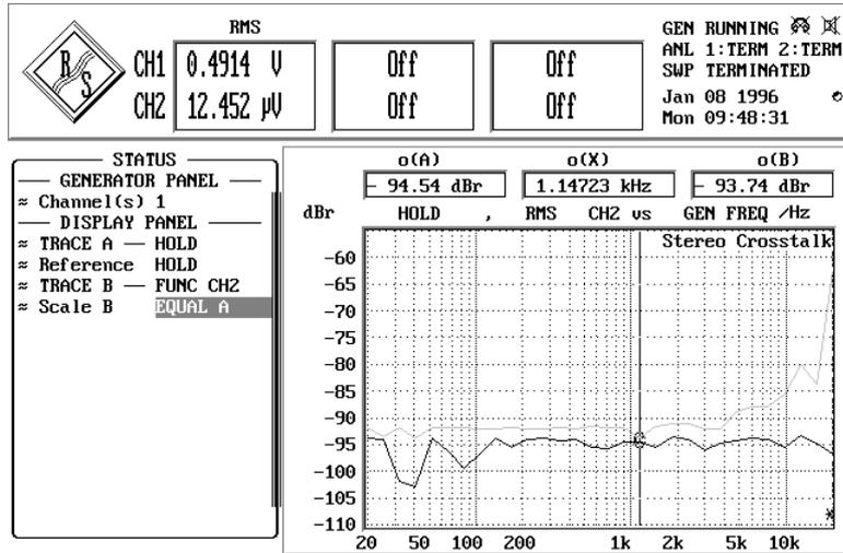
Fig. 2-29 STATUS and GRAPHICS panels with crosstalk measurement
