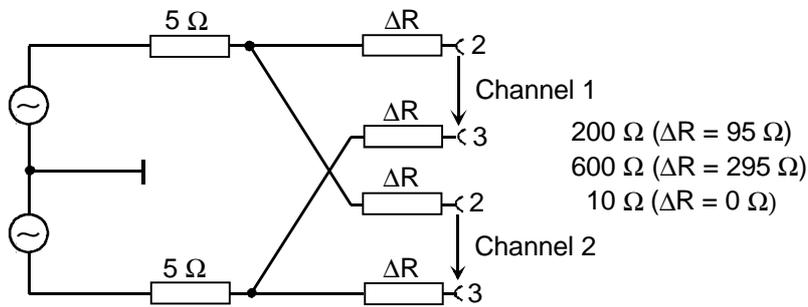
Fig 2-15 Balanced output
