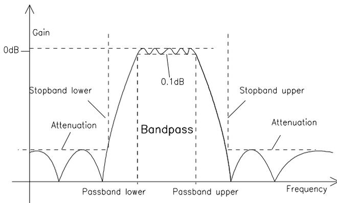
Fig. 2-34 BANDPASS frequency response together with filter parameters
