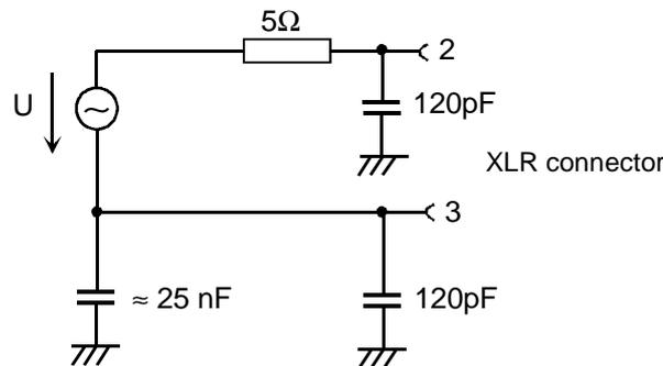
Fig. 2-12 Unbalanced output
