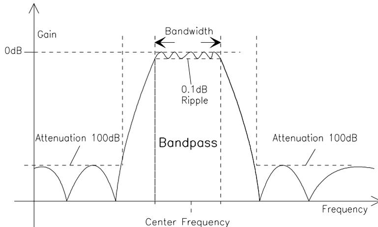
Fig. 2-21 Bandpass used for selective rms measurement
