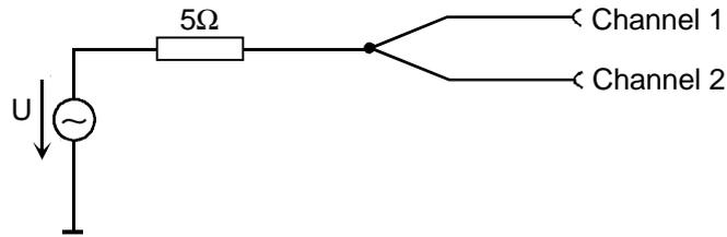
Fig. 2-13 Unbalanced output
