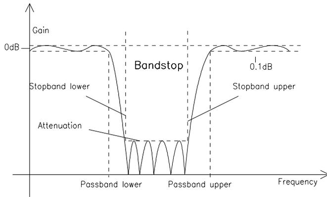
Fig. 2-35 BANDSTOP frequency response together with filter parameters
