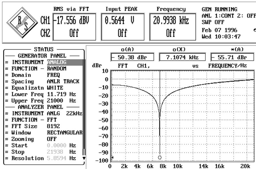
Fig. 2-32 Configuration and result of fast frequency-response measurement
