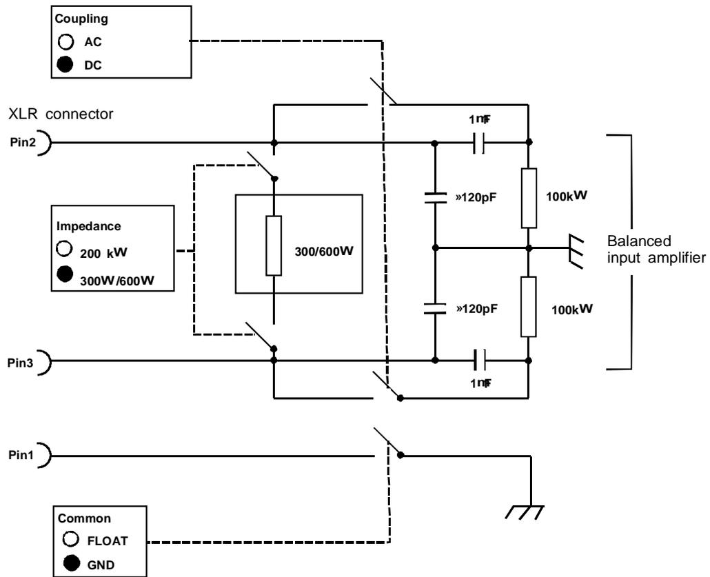
Fig. 2-16 Balanced input (Input BAL, channel 1 or 2)
