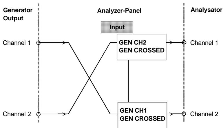
Fig. 2-19 Internal signal paths
