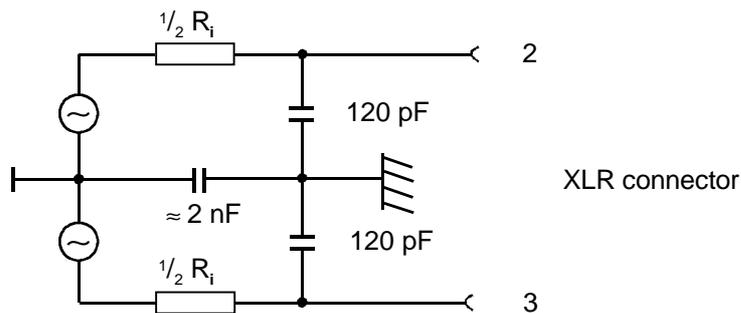
Fig. 2-14 Balanced output
