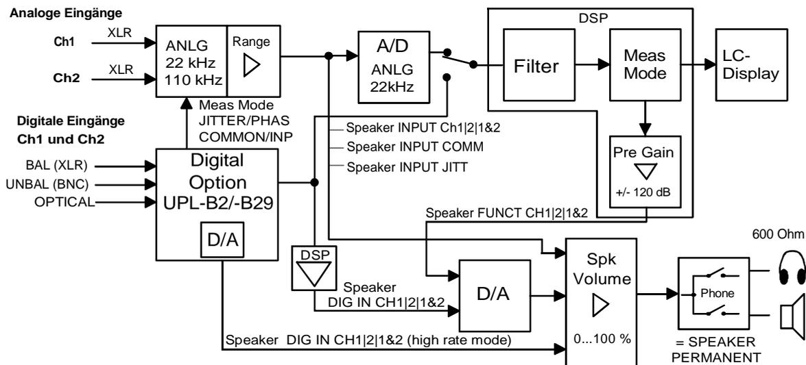
Fig. 2-28 Principle of operation of the headphones/speaker output
