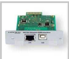
Ethernet/USB-interface H0730 for industrial use (Option)
