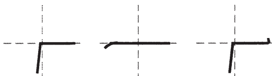
Type: Normal Diode Highvolt.-Diode Z-Diode 6.8V Terminals: Cathode-Anode Cathode-Anode Cathode-Anode Connections: (CT-GD) (CT-GD) (CT-GD)
