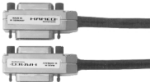
Figure 2: Shielded IEEE-488 round multiconductor
